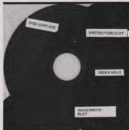
A 5¼" floppy disc with its protective envelope cut away.
